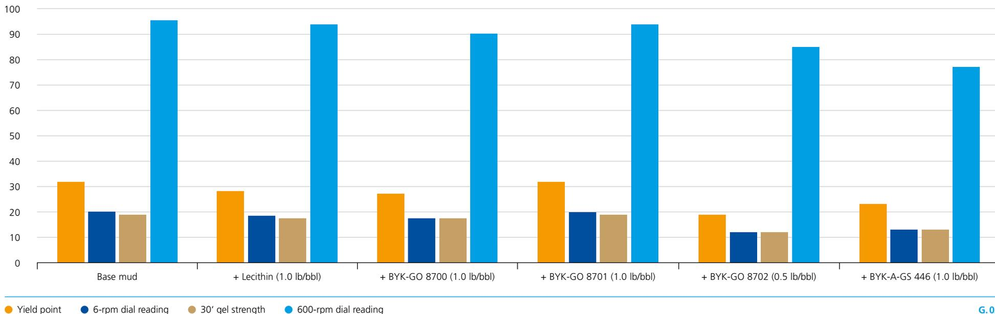
The drilling fluids were additionally heat-aged at 350 °F for 16 hours. Following the same procedure, rheological data were collected at 150 °F. After heat aging at this temperature, BYK-GO 8700, BYK-GO 8701, BYK-GO 8702 and BYK-A-GS 446 were found to be efficient thinners, each exhibiting temperature stability at 350 °F. The yield point, 6-rpm rheology, and 30-minute gel strength were consistent for each of the products.
