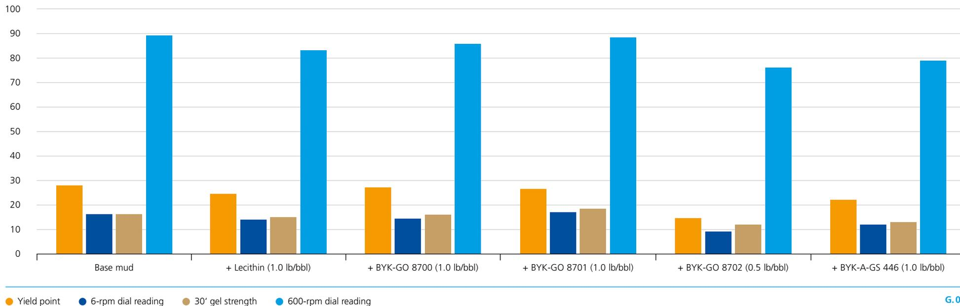
The muds were hot rolled at 250 °F for 16 hours and tested again at 150 °F. BYK-GO 8700 and BYK-GO 8701 both performed equally as well as lecithin. At 250 °F, BYK-GO 8702 and BYK-A-GS 446 again conditioned the mud to optimal rheological ranges.
